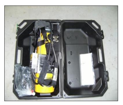
Each swabbing rig is equipped with two 30 min self-contained breathing apparatus. Swab Master Ltd. uses the Scott 2.2 self-contained breathing apparatus shown here.
